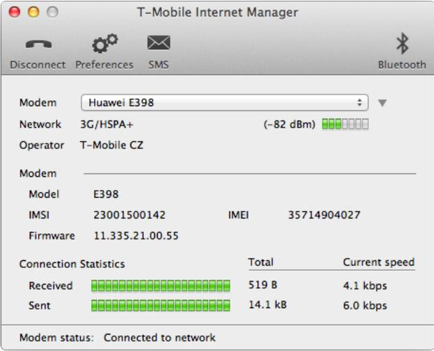
When a connection is active, the button with receiver changes its appearance to a replaced handset. Clicking this button will terminate the connection.
