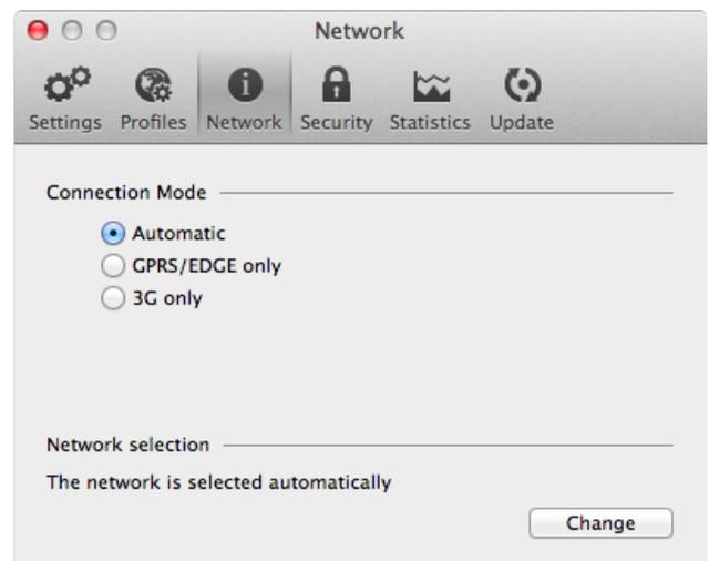
The automatic network selection and connection mode is selected by default. Click the Change button to change the network. A list of currently available networks is presented. Select the particular network you want followed by the OK button. The device will connect using only this service provider.
