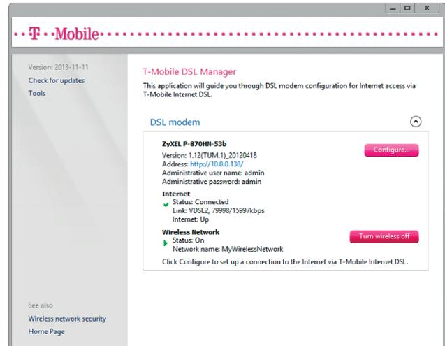
The status of the wireless network will change to „Off“. When you later want to turn the wireless network back on, click **Turn wireless on**.
